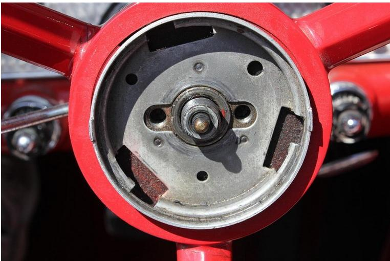
Here is a view of the original steering wheel hub after the lock nut was removed. You can clearly see the horn button contact in this photo.
