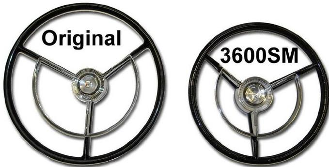
The 3600SM smaller steering wheel is a solution for those 1956/57 T-Bird owners who desire some extra wiggle room from the driver's position. The 3600SM is a scaled down reproduction steering wheel with matching horn ring that is 2" less in diameter than a stock 1956/57 Thunderbird steering wheel.
