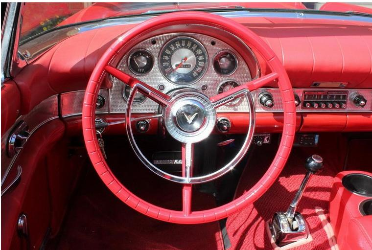
Carefully place the 3600SM steering wheel on the shaft and make sure the “smooth” 1/3 of the wheel is on top. Press down and wiggle with moderate pressure to start the wheel on the shaft. Install the center nut and tighten with a 15/16” socket until the steering wheel is fully seated. Wiggle it to ensure that there is no play. Lock the new horn ring in place by pressing down and twisting it clockwise until it snaps into position. Reconnect the battery and test the horn.
