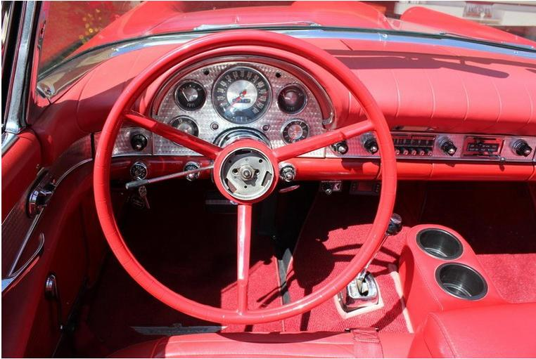
This photo shows the original steering wheel after the horn ring was removed. You can see the 15/16" nut that fastens the wheel to the shaft and a little metal button in the center of the nut, which is attached to the horn relay wire.
