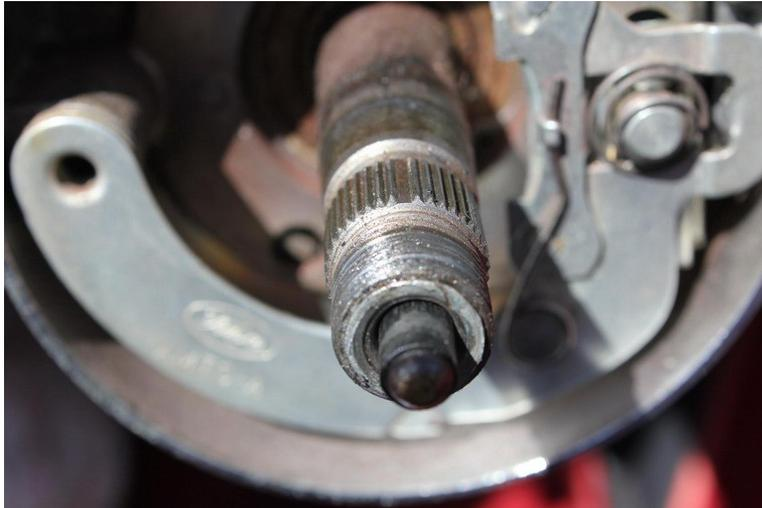
This close-up view of the steering wheel shaft shows that the shaft is keyed with a wider groove at the top of the assembly. This wide groove mates with a corresponding wider key on the steering wheel hub. The original wheel can only fit on the shaft one way.
