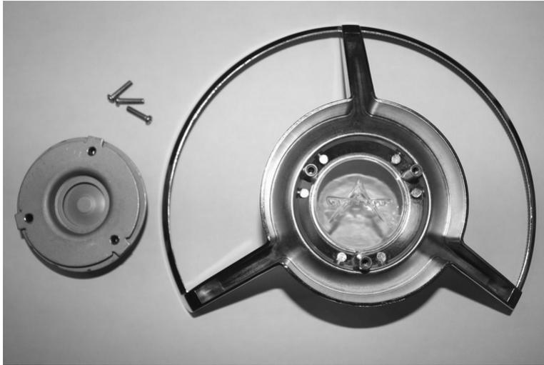
This is a view of the disassembled horn ring with the generic emblem still in place. This emblem can be removed and discarded. It will be replaced with a correct Ford emblem during the reassembly process.
