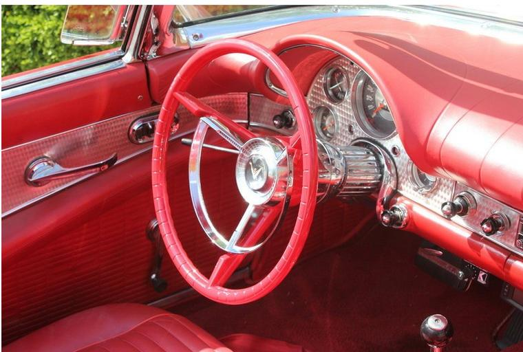
Here is the new steering wheel shown from a slightly different angle. It looks quite authentic. You can see that there is now significantly more space between the bottom of the steering wheel and the seat. The driving position is much more natural using the smaller steering wheel, especially for larger drivers.
