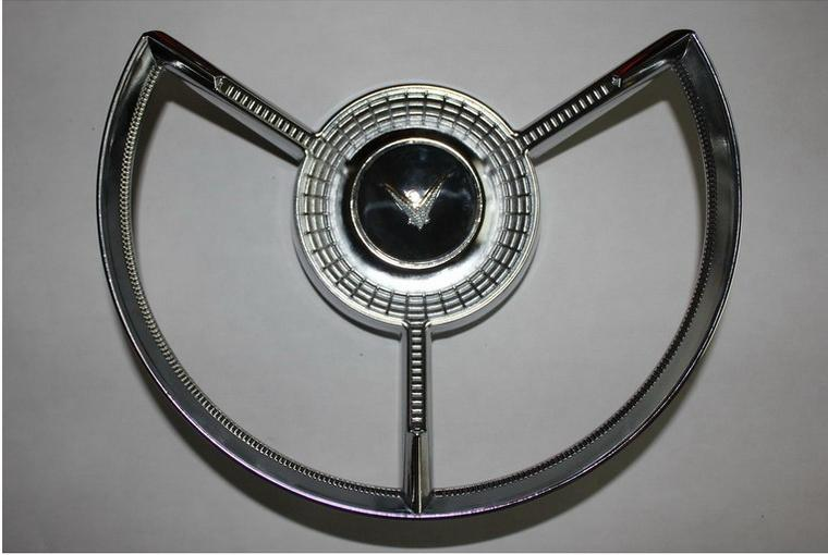
Flip over the horn ring and it should look like this photo. Other than the smaller size, the only thing that distinguishes the 3600SM horn ring from some originals is that it lacks the “Ford Master Guide Power Steering” legend under the hub. Ironically, the smaller steering wheel is probably only appropriate for those cars that actually HAVE power steering, but basing the repro horn ring on a manual steering car avoids Ford licensing issues.
