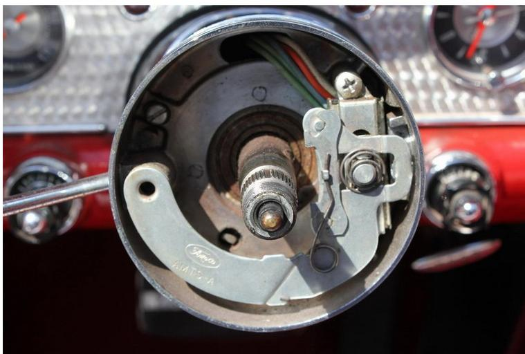
This is the steering wheel shaft and turn signal switch assembly after the original steering has been removed.
