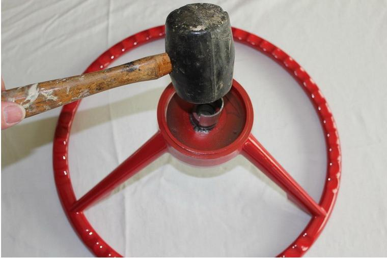
The new turn signal sleeve should fit tightly around the 3600SM steering wheel hub. If the sleeve snaps easily onto the hub and can be rotated using only moderate finger pressure—it is too loose. Remove the sleeve and carefully squeeze it in a vice to reduce the diameter slightly. Then carefully tap the sleeve onto the shaft with a rubber hammer. Once in place, use the large pliers to twist it into final alignment, using the original steering wheel as a reference.
