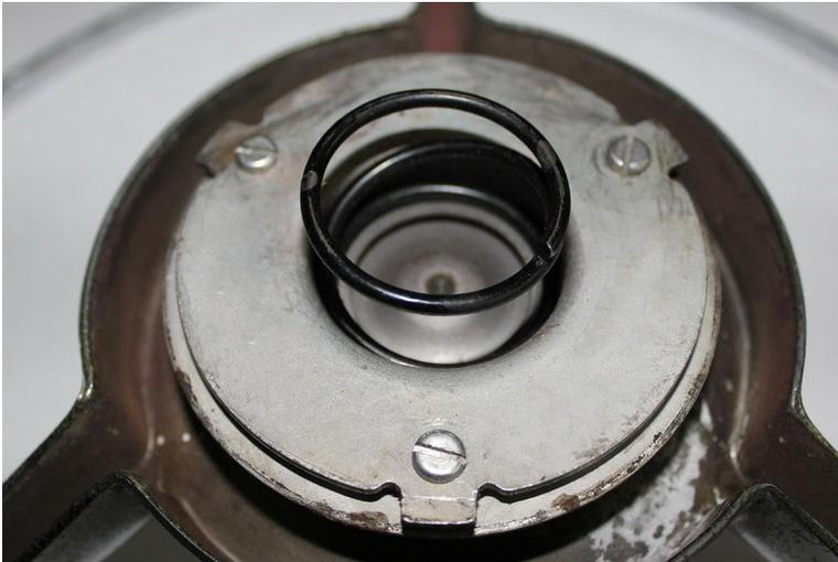
The back of the original T-Bird horn ring shows the horn ring spring. This part, CASCO No. [13A807](#), is not included with the 3600SM smaller steering wheel, so be sure to order one from CASCO when you buy the new steering wheel. This way you can store the original steering wheel as an intact unit, complete with center medallion and horn ring spring.
