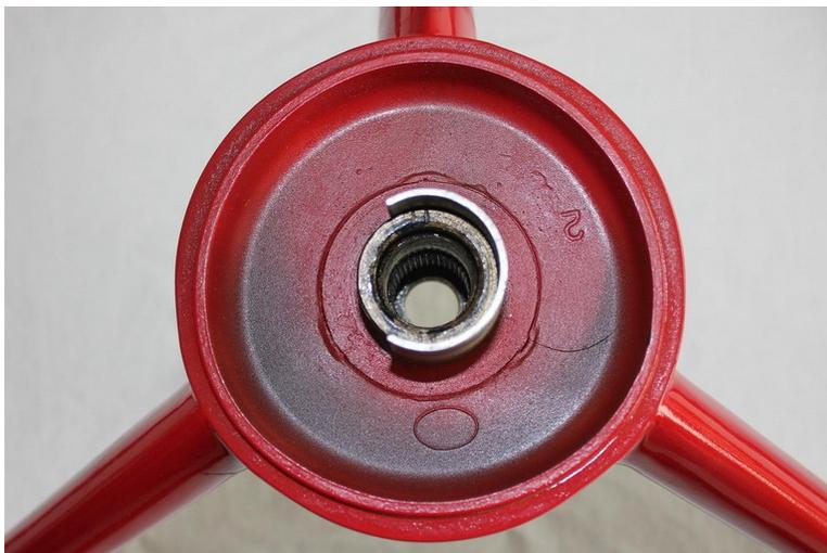
Here is another view from directly overhead. Position the new 3600SM steering wheel directly below the original steering wheel so you can install the half-round sleeve on the new wheel in the exact same position.
