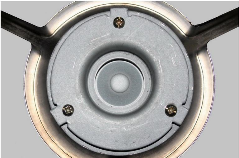
While the wheel is out being painted, it is a good time to install a correct 1956 or 1957 T-Bird emblem in the horn ring. To do this, flip the ring over and remove the three Phillips head screws.
