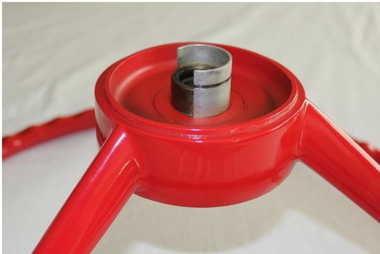
This is a view of the rear hub of the original steering wheel. You can see the half-round silver sleeve that is used to cancel the turn signals.
