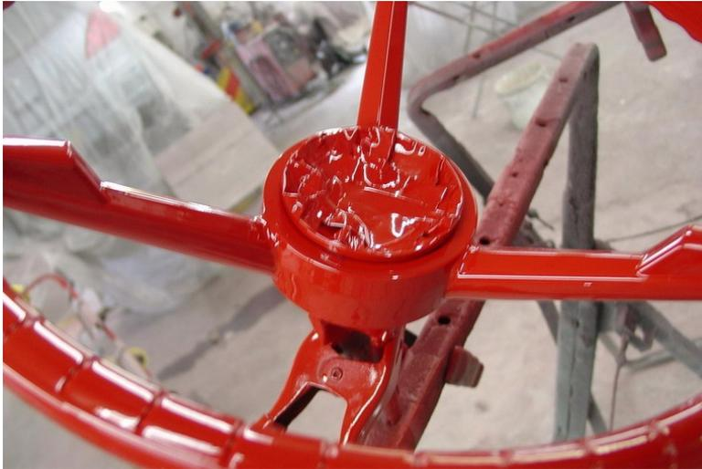
Remove the horn ring by pressing down evenly and then giving it a counter-clockwise twist. Retain the horn ring while the steering wheel is painted.
