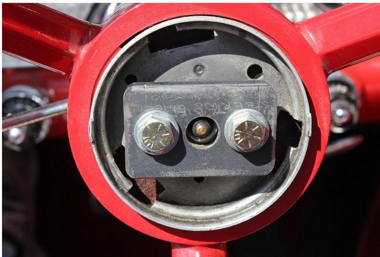
Here is the steering wheel puller in place, ready to do its duty. Each hex bolt is gradually tightened using a 1/2" socket wrench. Once one bolt feels tight, move to the other. Eventually the steering wheel will be loosened on the shaft and can be easily removed by pulling it toward you.
