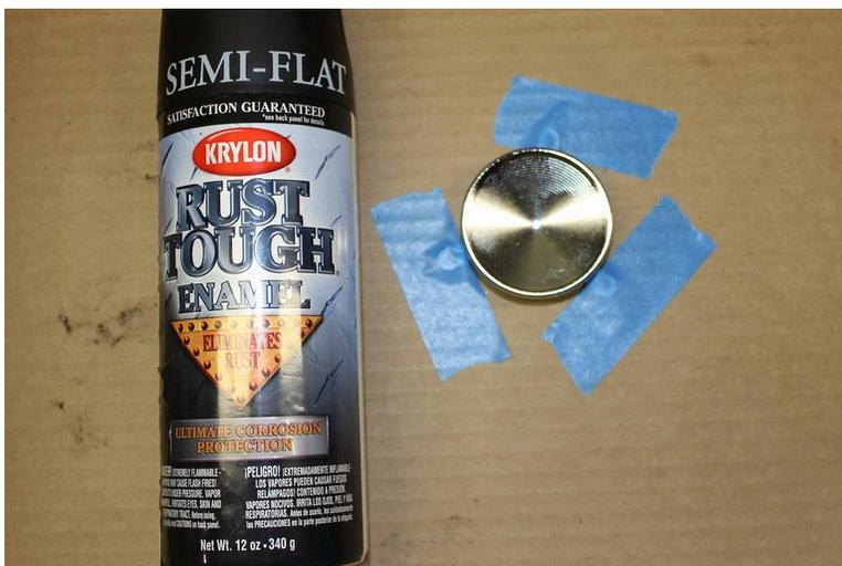
The other part of the horn ring assembly is a round conical-shaped trim piece that is mounted directly behind the center emblem. If your T-Bird is a 1956, the supplied silver color is correct. The example car was a 1957, so it was necessary to paint this piece black. Carefully scuff the surface with steel wool, clean it with solvent, primed it and then painted it. Semi-flat black spray paint from a rattle can works fine.
