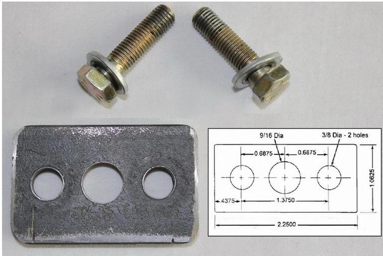
This is the steering wheel puller that was made from a diagram published in Issue 10, October 1997 of CASCO's ThunderEnlightening newsletter. A piece of 1/4" thick steel bar stock and a drill press are used to make the custom puller. The large center hole is critical, because it enables the horn button wire to poke through without being damaged. The two hex bolts are 5/16-24 (fine thread), 1-1/4" long.
