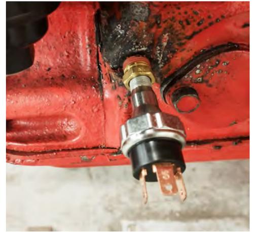
Remove the hex socket head plug in the oil rail located nearest the fuel pump as shown. In the example pictured some heat was required to persuade the plug to let go.
