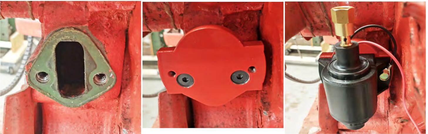
Start the installation by removing the original fuel pump. Save the 90° fitting and the flexible fuel line to reuse with your new electric pump.
