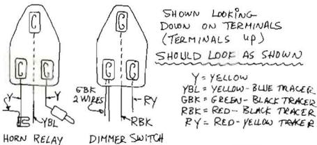
The plugs should look like those in the sketch. We have found the center terminal to be ok but the two outside terminals to be reversed. This problem can be fixed by either cutting the wires or by slicing open the plug, switching the terminals, and gluing and plug back together.
