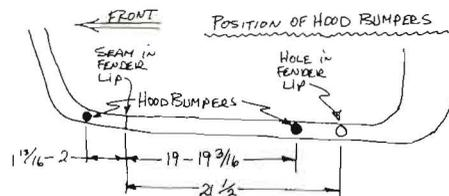
□ **Position of Hood Bumpers** 1955 T-Birds did not come from the factory with hood bumpers but both 56's and 57's did. This sketch shows where the bumpers were located. The variation in dimensions is variation measured on original unrestored cars. All dimensions are in inches.
