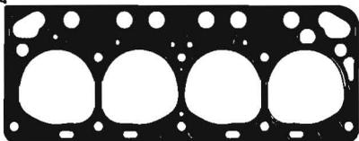
□ **Head Gaskets** If your engine has been rebuilt lately and it seems to be running hot check to see if the head gaskets were installed properly. All y-block head gaskets are made with three rounded corners and one square corner. The square corner MUST be at the upper front on both sides of the engine for proper coolant flow.
