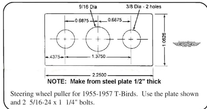
❑ Removing the steering wheel requires a puller to break it free from the shaft. If you have access to a drill press you can easily make the puller above to do the job (see sketch). The 1/2" hole in the center is for clearance for the horn wire. Don't skimp here and leave this hole out, unless you remove the horn wire you will damage it!
